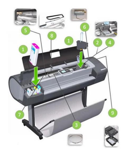
1. Print heads have 200 microscopic nozzles firing ink droplets so fine that it forms an aerosol mist. Some of this ink mist is suspended above the paper and with each carriage pass is pulled into the finer workings of the Design Jet, depositing a thin layer of ink throughout.
